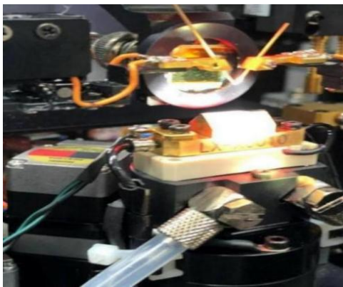
Test chuck with high heat dissipation high-abrasion, as well as optical detector and optical coupling system
