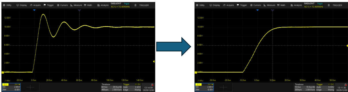
Waveforms Comparison Before and After APFC Adjustment
